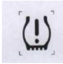
Figure 3: Tire Pressure Fault Symbol
